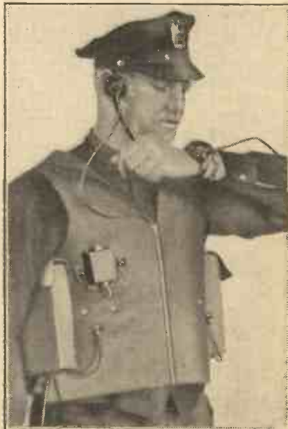
THE "RADIO VEST," developed by R.C.A. for the use of the police, fire and other services, is a complete U-S-W transmitter-receiver.
